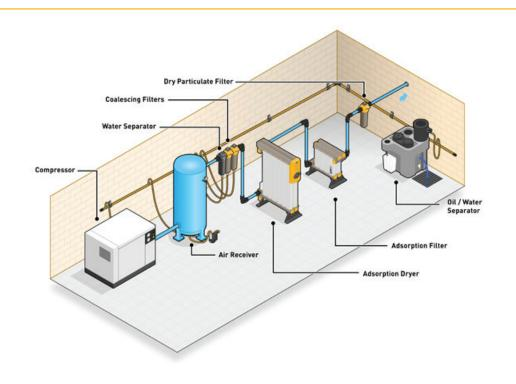
Heatless adsorption dryers (also known as PSA dryers) are the simplest type of adsorption dryer available and have long been the dryer of choice for many industries and applications. They are simple, reliable and cost effective and for small to medium flow systems, often the only viable technology available. Additionally, modular heatless dryers provide an even more reliable, smaller, more compact & lightweight dryer which can be installed in both the compressor room or at the point of use.
