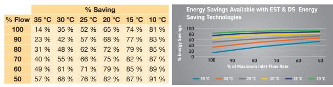
Example based upon a CDAS HL 075 / OFAS HL 075 Purification System and referenced to a 3 Minute Standard Cycle. Energy savings are applicable to all CDAS / OFAS / FBP / MXS-DS / MXLE models.
